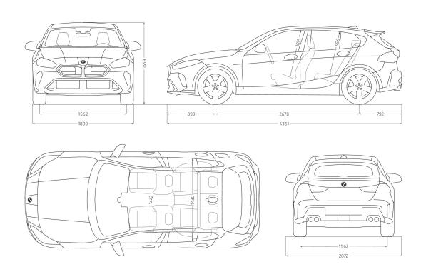
The dimensions in the technical drawing are in millimetres and may vary depending on the model and the optional equipment.
