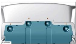
8. Remove push pins (x13) securing front underbody cover to front subframe and remove front underbody cover.
