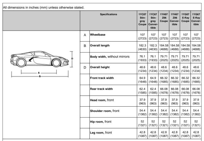
Published dimensions indicated are without optional equipment or accessories. Additional accessories or equipment ordered at the customer's request can result in a minor change in these dimensions.
