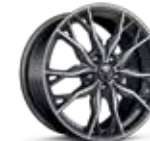
20-spoke bright machined-face After Midnight-painted forged aluminum wheels: 19" x 8,5" J front and 20" x 11" J rear (Q99)
